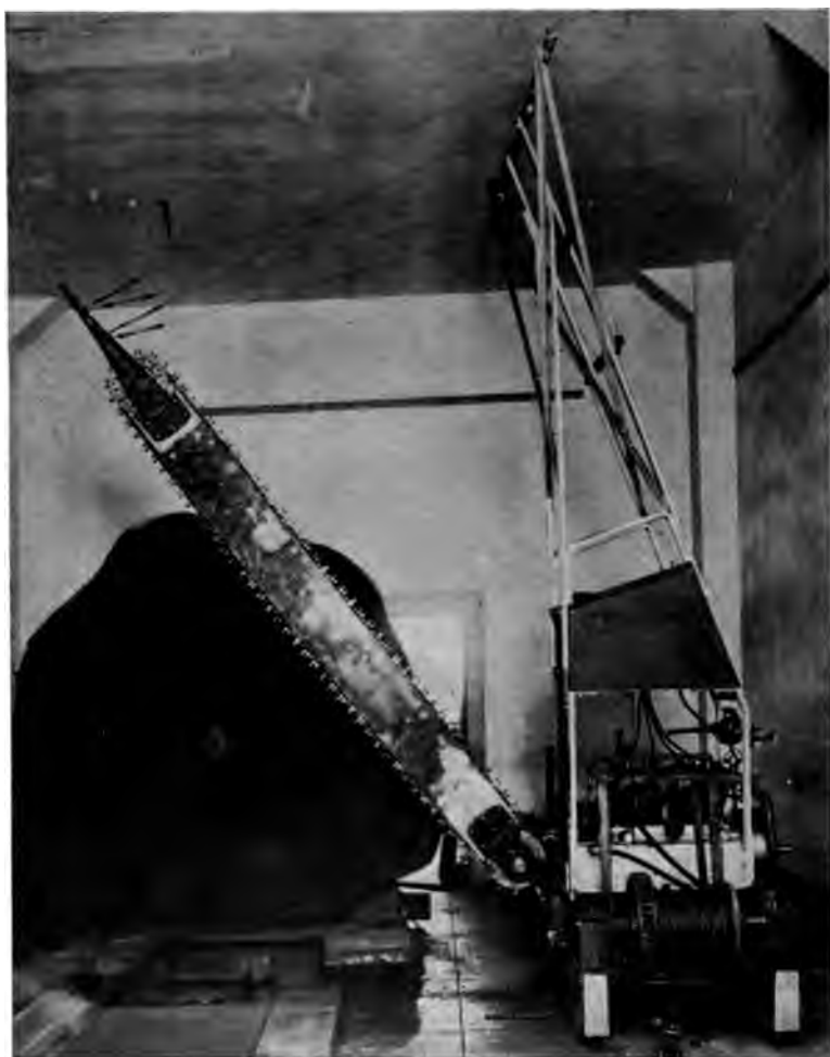
FIG. 16. -- The Endless Chain Saw used in Bucking-up Logs in the Pacific Coast Forests.
